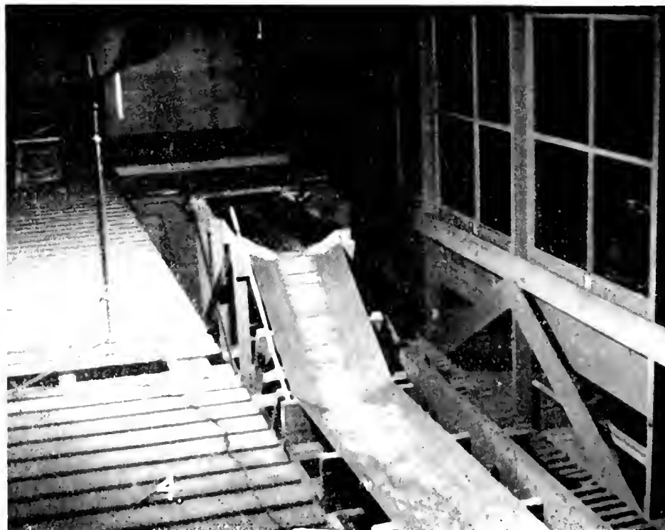
Same dissipating basin dimensions as Fig. 3. Flow is equivalent to 900 c. f. s. in prototype
